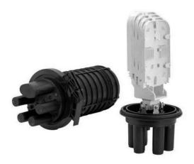
Splice Joint Closure is a device use to provide space and protection for fiber optic cables that are spliced together. The Splice closures are designed for use with any cable construction (Loose Buffer tube, Central core tube, Loose fiber and Ribbon fiber). These closures can be installed on Aerial, Pedestal, Underground buried, Handhole, Manhole and Pole mount
